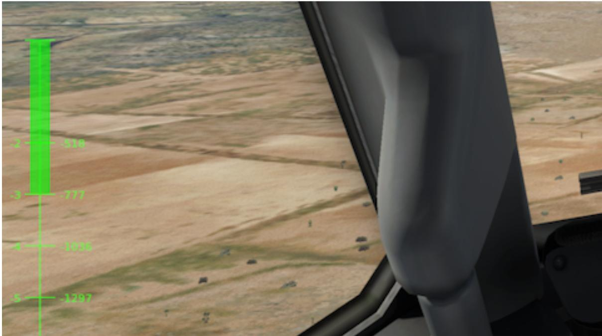
Figure 7: Detail of the opening figure, showing the actual vertical speed in relation to the vertical speed required for a glide slope angle between 2° and 5°.
